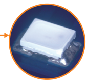
Chip components are mounted on PET film with low temperature soldering
