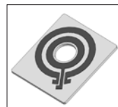
Printed resistance on PWB 抵抗印刷基板
